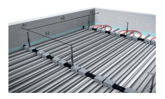
a1: max. 400 mm a2: max. 1280 mm b1: max. 150 mm b2: max. 800 mm
